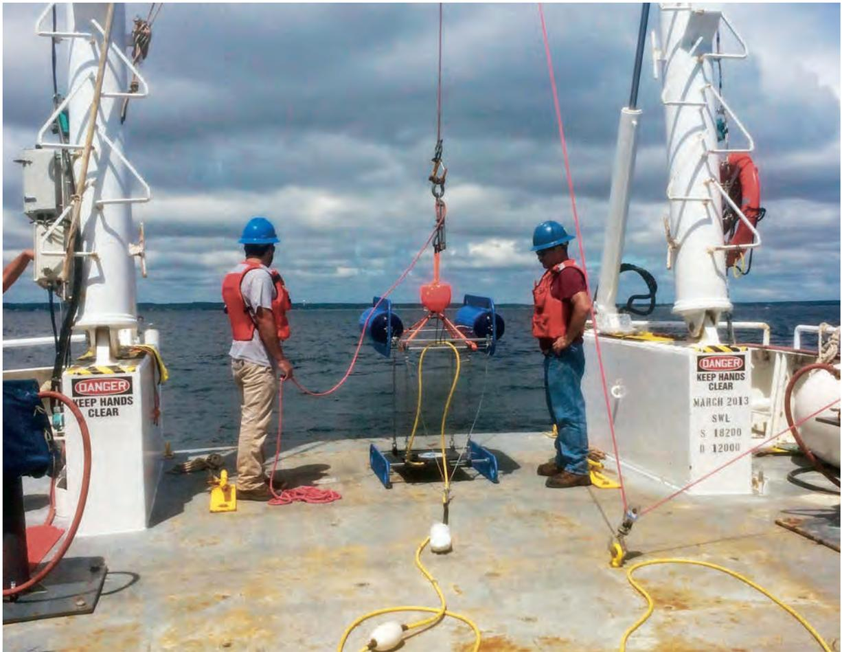
**Researchers prepare to deploy a seismic “bubble gun” to survey the sand and gravel deposits on the sea floor. This tool uses a low-frequency signal that can penetrate through coarse sand and gravel to produce high-resolution images of seafloor sediments. This method helps locate pockets of sand and determine their volume.**
