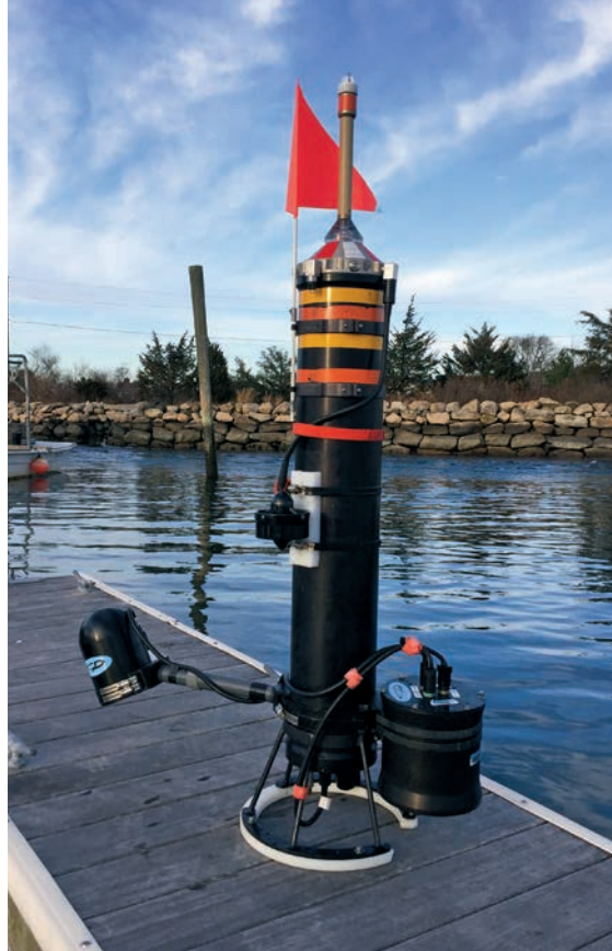
This photofloat delivers high-quality, low-cost images of the seafloor. Photograph courtesy of Christopher Roman
